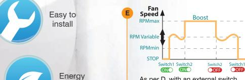
As per D, with an external switch for operation at RPMmax.
